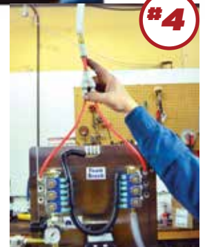
Attach one end of manifold to the air feed, the other to the chemical feed. Run from manifold to bays with Polybraid Hose. Repeat for each solenoid set.
