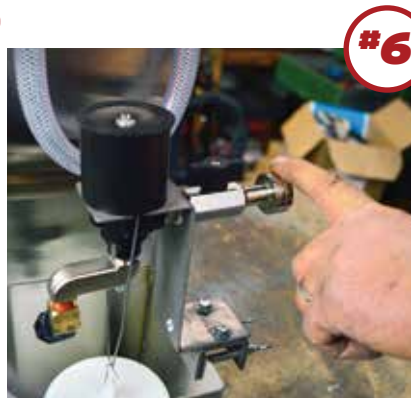
Now you are ready to hook up the water source to the Hydrominder. Then put the soap pick up tube from the Hydrominder into the chemical.
