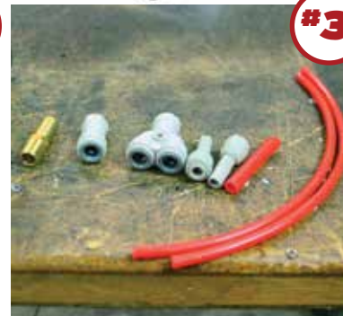
Now it's time to plumb the unit to feed the chemical to the bays. Tom creates his own manifold using the following: 1: JG6DV 2: JG6R4 1: JG6FC4 1: BFA29-84 1/4" Polytubing
